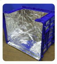
**STEP 5** Line the inside of the two crates with foil.
