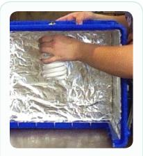
**STEP 7** Gently screw the 150-watt equivalent, 40- or 42-watt CFL bulb into the hole from inside the crate.
