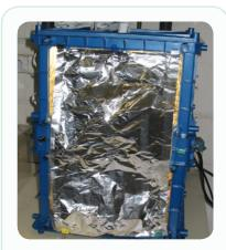
**STEP 12** Make a foil curtain to reflect light back into your Light Box by reinforcing a sheet of aluminum foil with scotch tape.
