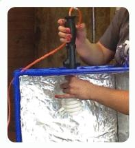
**STEP 9** Thread the drop light onto the bulb from outside the crate.
