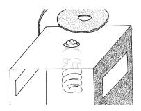
5. Insert the light fixture through the hole inside the box.
